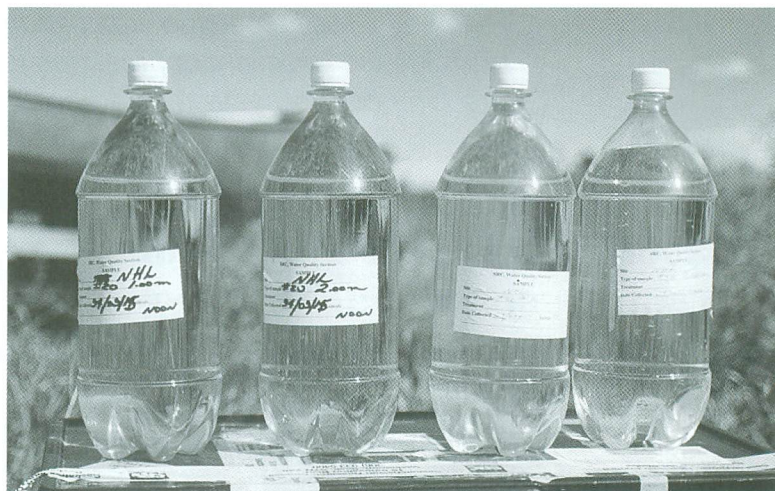
Brown water (bottle to the left) before coagulation treatment turns crystal clear (bottles to the right)
