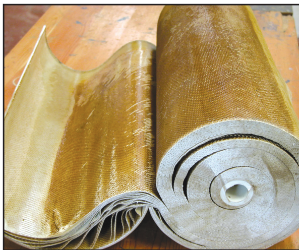
RO membrane after manganese greensand treatment at George Gordon First Nation, 2004, before the IBROM was installed. A membrane that is new or has not been fouled is white. SUBMITTED PHOTO
