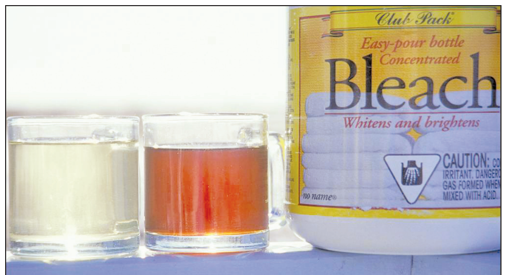
The photo shows two cups of tea. Into one serving chlorine has been added. However, organic material from the tea reacts with chlorine to form trihalomethanes.
