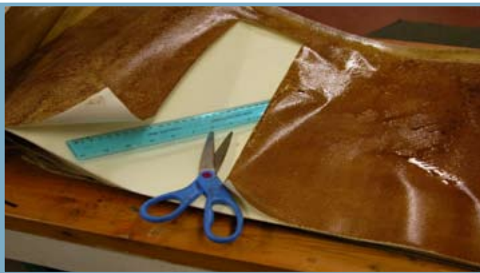
Fig. 3. A cut open reverse osmosis membrane fouled by manganese oxidizing bacteria leaving a brown coating on top of a bright white membrane sheet. From the George Gordon First Nation water treatment system.
