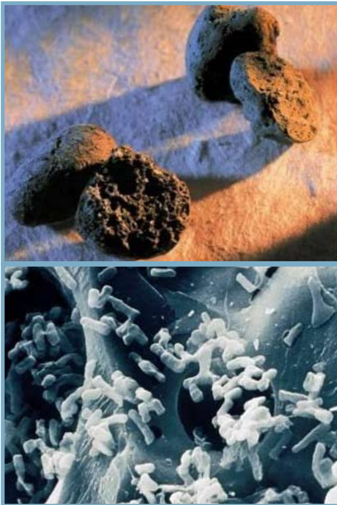
Fig. 5. Upper: Expanded clay material (Filtralite) with size similar to coarse coffee grounds. Lower: Electron microscope photograph showing bacterial clusters on the expanded clay material.
