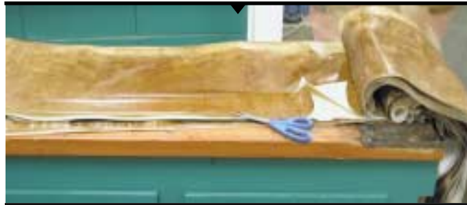
Pieces of RO membrane that were fouled by manganese greens and treatment.
